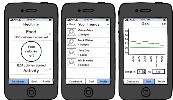
Fig. 3. Homescreen, screen with the badges earned by friends and screen with a visualization of the weight of the user through time, as they were in the first paper prototype
